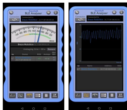
Figure 9: Third-party Application showing the stats of the BLE beacons at 1 meter away.
