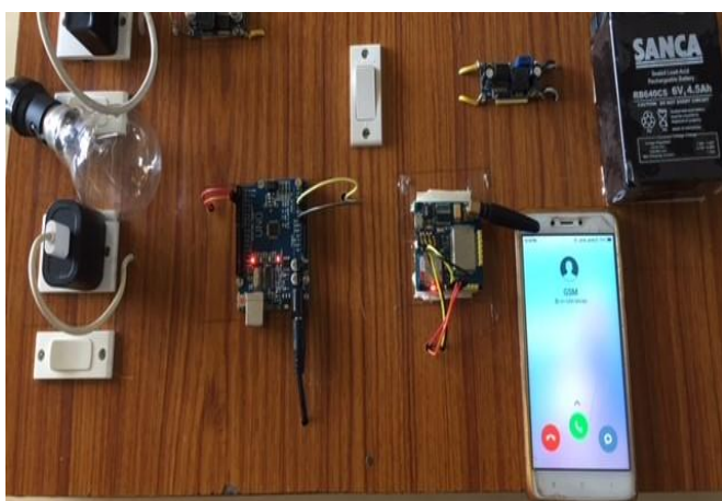
Figure 5: Intimating call from GSM when the absence of power supply
