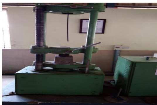
Figure 3: Test for compressive strength using UTM
