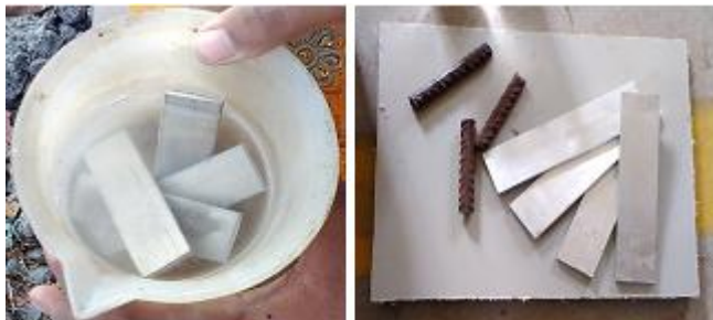
Figure 1: Metal Samples coated with corrosion inhibitor
