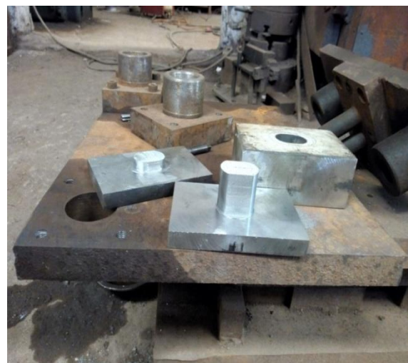
Figure 1.1: Die, Top & Bottom punch
