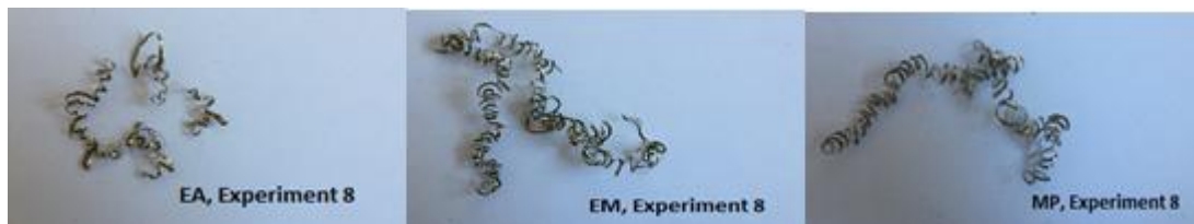
Figure 4: Images of chips formed by cutting tools with different chipbreaker forms when machining
