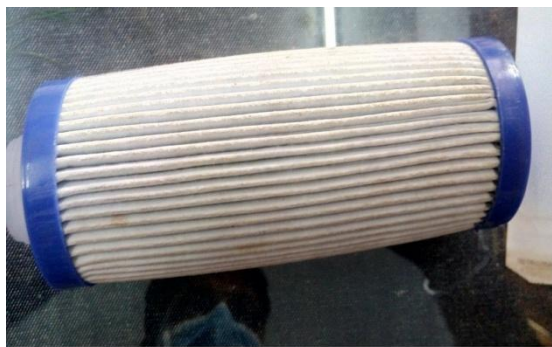
Pleated form of the 6 layered cartridge
