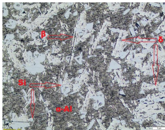
**Figure 2:** Optical microscopy micrographs of AICC2 (Al-Si-Fe-Nb-Ni)
