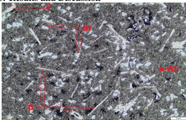
**Figure 1:** Optical microscopy micrographs of AICC1 (Al-Si-Fe-Nb)
