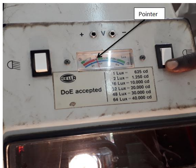
Figure 3-1: Beam setter reading after correction was at “green” between 16-32 lux
