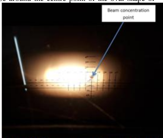
Figure 3-2: Beam concentration around the point before adjustment
