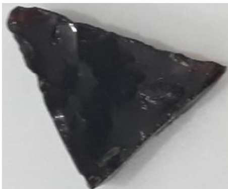
Figure 10: Sample Hp-2 fragment photo of the vitrified heterotermopolymer of copaiba oil-resin (COR) using the vitrification protocol 2.
