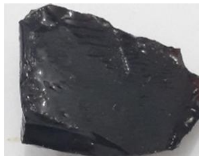
Figure 13: Sample Hp-3 fragment photo of the vitrified heteropolymer of copaiba oil-resin (COR) using the vitrification protocol 3.
