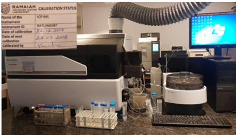
INDUCTIVELY COUPLED PLASMA MASS SPECTROPHOTOMETER (THERMO FISHER SCIENTIFIC GMBH, BREMEN, GERMANY) SAMPLES KEPT FOR DIGESTION
