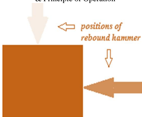
Figure 5.5: Positions of rebound hammer
