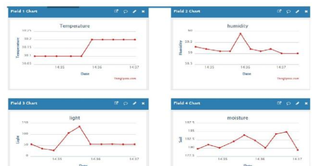
Figure 5: Snapshot showing variation of graph of sensor values of Laterite soil using ThinkSpeak application.
