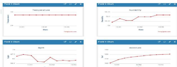
Figure 5: Snapshot showing variation of graph of sensor values of Laterite soil using ThinkSpeak application.
