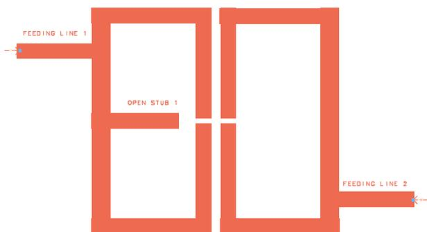
Figure 2: Layout of open loop stub loaded resonator
