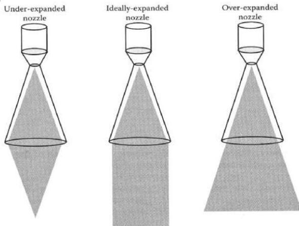
Figure 2: Nozzle Geometry
