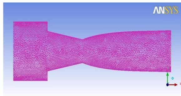
Figure 5: Mesh file of rocket nozzle
