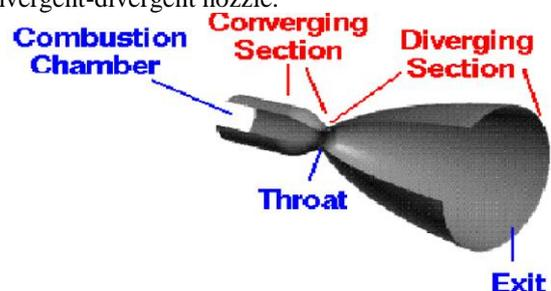
Figure 1: Parts of rocket nozzle
