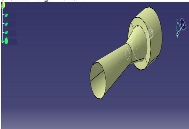
Figure 3: Catia design of rocket nozzle
