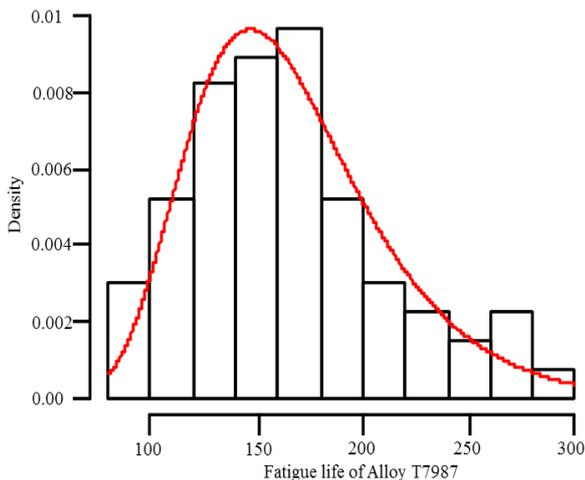
Figure 5: E-epsilon distribution plots of Alloy T7987 fatigue life (in thousand cycles)
