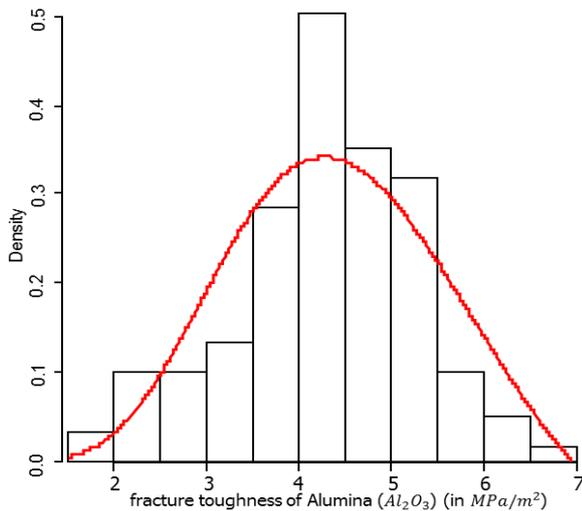
Figure 4: E-epsilondistribution plots of fracture toughness of Alumina
