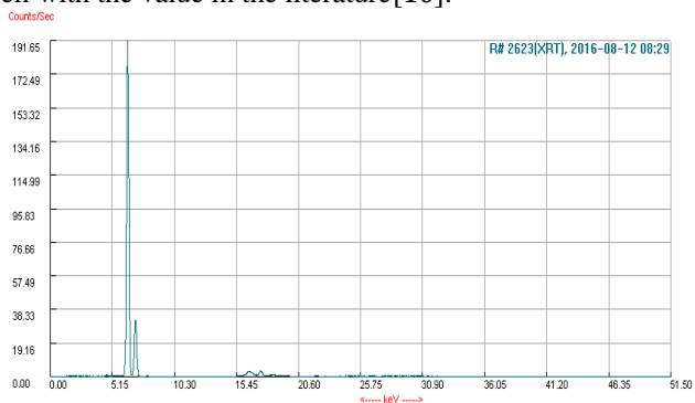
Figure 5: XRF spectrum of Magnetite sample
