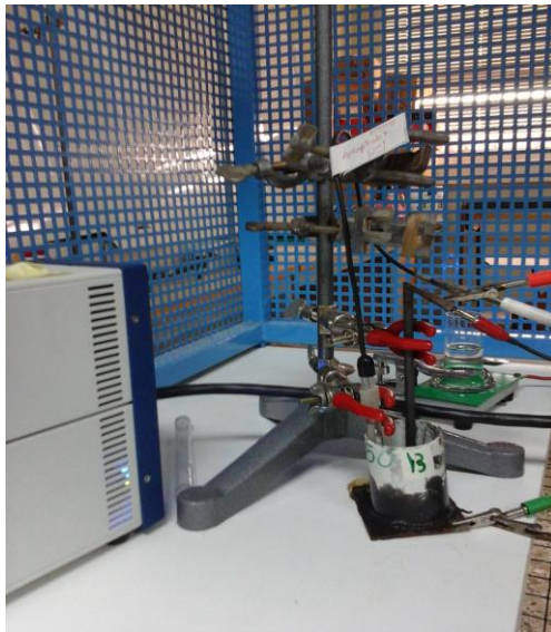
Figure 2: Experimental setup for impedance measurement
