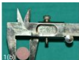
Figure 1 (a): Circular disc specimen of thickness 2mm
