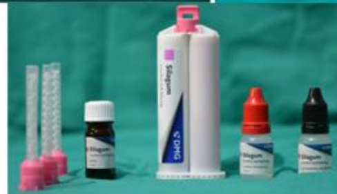
Figure 3: Room temperature vulcanized silicone soft liner (Silagum Comfort, DMG, Hamburg, Germany) applied on one of the surfaces in thickness of 2mm making the total thickness of the specimens as 4mm and the nature of the interface between the denture base resins and silicone soft liner were observed under the Scanning electron microscope
