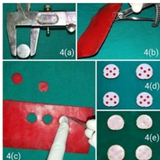
Figure 4(a): 16mm circular metal disc templates; Figure 4(b): Modelling wax of thickness 2mm; Figure 4(c): Circular wax patterns being cut from modelling wax of
