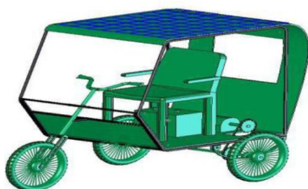
Figure1: Prototype of a tricycle powered by solar energy Source: Designing Solar Three-Wheeler for Disable People /Md. Shahidul Islam, Zaheed Bin Rahman, Nafis Ahmad/ International Journal of Scientific & Engineering Research Volume 3, Issue 1, January-2012 ISSN 2229-5518
