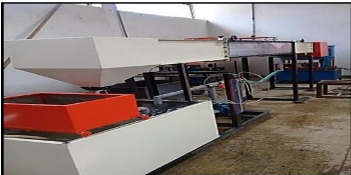
Figure 3: Rectangular open canal flume set up (Hydraulic Laboratory, Purwanchal campus , product of Arm field company, UK)
