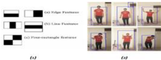
Figure 1.2: (1) shows the Haar filters used as Cascades, (2) Shows the body detect output after applying Haar cascades on dataset
