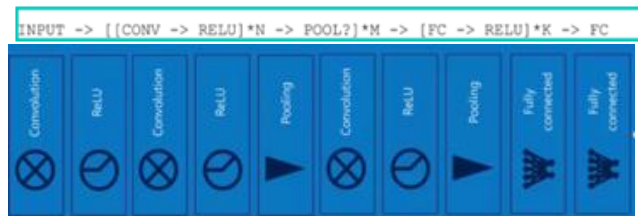
Fig 1.8 Graphical representation of a Layered CNN Architecture
