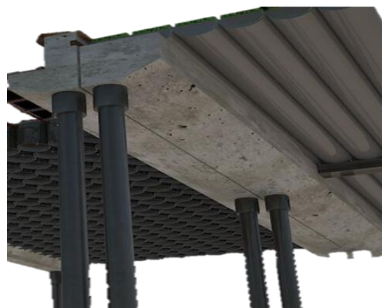
Figure 19: Perspective shot of the use of pipes as basins for planting
