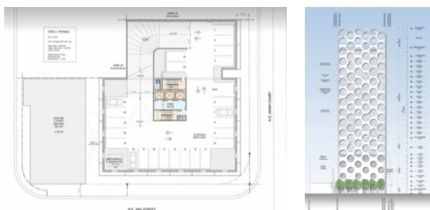
Figure 3: COR Building, the parking level and the elevation view of perforated shell
