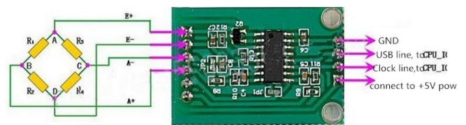
Connection method between load sensor and HX711 load module Figure 8: Connection method between sensor and Hx711 module
