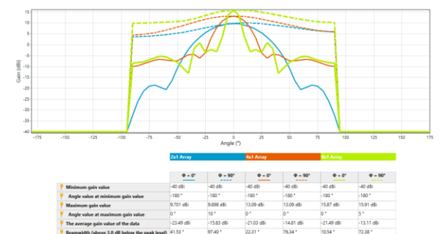
Figure 18: Gain (dBi) vs Angle (°) at 5 GHz for 2x1, 4x1, 8x1 Rectangular Patch Array
