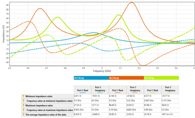
Figure 12: Impedance (Ω) vs Frequency (GHz) at 5 GHz for 2x1, 4x1, 8x1 Rectangular Patch Array
