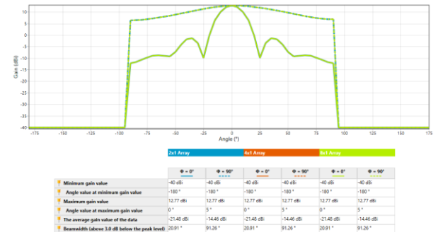
Figure 17: Gain (dBi) vs Angle (°) at 2.45 GHz for 2x1, 4x1, 8x1 Rectangular Patch Array
