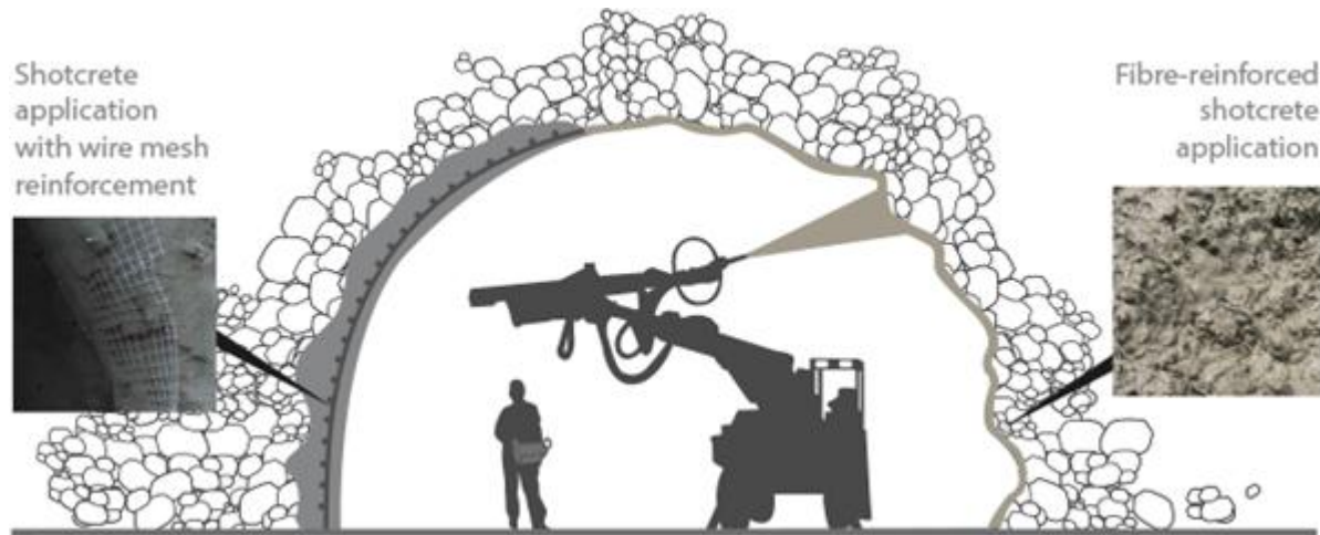
Figure 11: Steel fiber-reinforced shotcrete (SFRS) [93]
