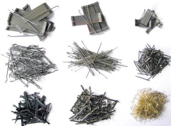
Figure 2: Types of steel fibers [20]
