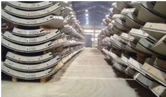
Figure 12: Segmental tunnel lining using steel-fiber-reinforced concrete [93]
