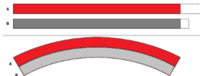
Figure 3: Bending of bimetallic strip on change in temperature
