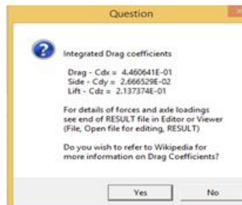
Figure 14: Spot values, % error - cut off and drag coefficients at 70mph velocity
