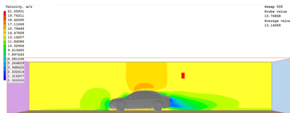
Figure 15: Velocity distribution at 30mph
