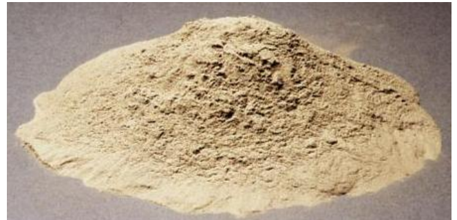
Figure 1: Fly ash, a powder resembling cement, has been used in concrete since the 1930s. (IMG12190)
