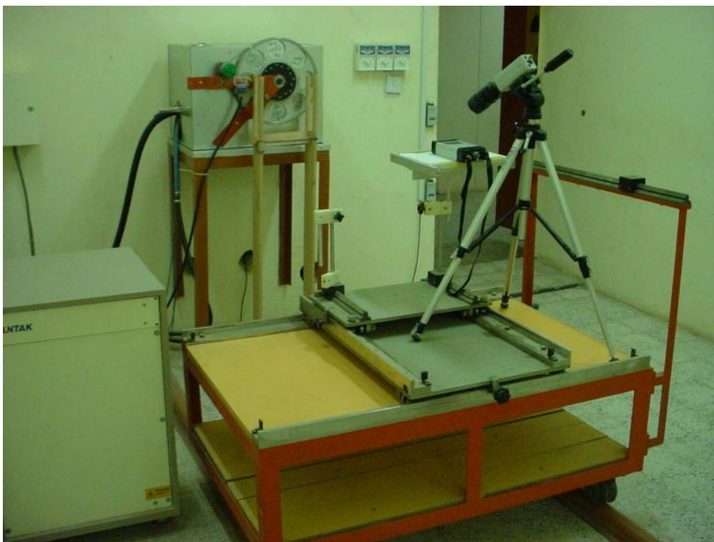
Figure 2: Set up for the calibration of a survey meter at the Secondary Standard Dosimetry Laboratory.
