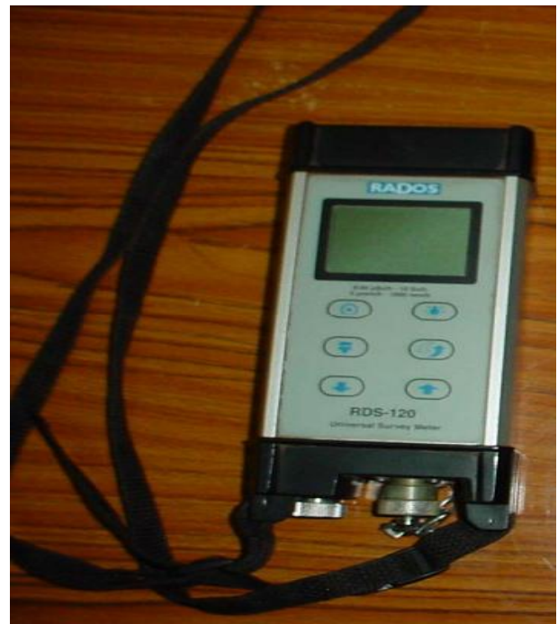
Fig .1: A typical universal survey meter(Rados-120)
