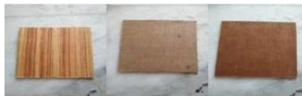
Figure 1: Natural fiber insulating panels (Sisal, Flax, Jute)
