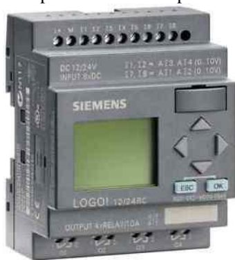
Figure 6: Programmable Logic Controller (PLC)
