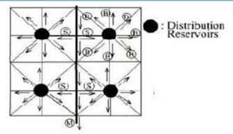
The area is divided into different zones. The water is pumped into the distribution reservoir kept in the middle of eachZone. The supply pipes are laid radially ending towards the periphery.
