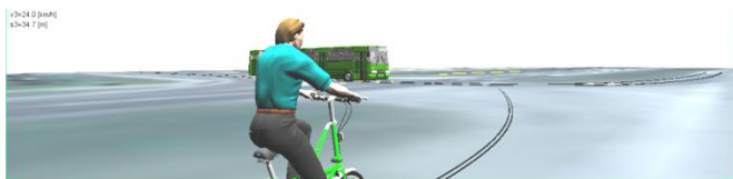
Figure 8: Reciprocal positions of the bus and bicycle at the time the bus was at the junction border, according to the position indicated by cyclist
