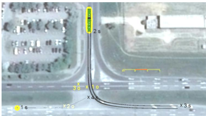
Figure 7: Reciprocal starting positions of the bus and bicycle according to the position indicated by cyclist (in ground plan)
