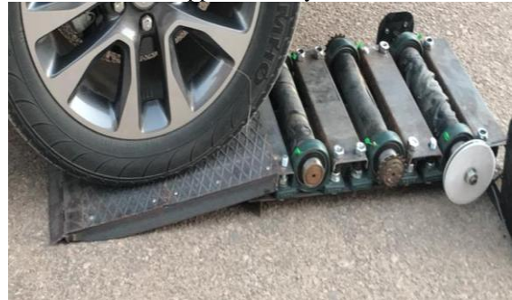
Figure 11: Roller system implemented and prepared for Car experiments
