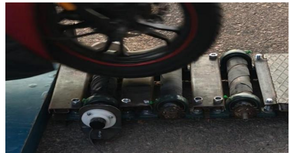
Figure 12: Roller system implemented and prepared for Motorcycle experiments
