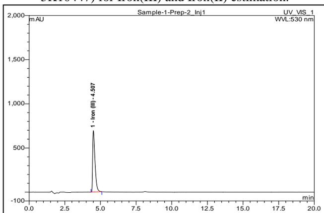
**Figure 3:** Iron Polymaltose sample chromatogram (B. No. 238062) for Iron(III) and Iron(II) estimation.
