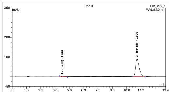
Figure 3: Specificity chromatograms for Iron(III) (10mg/L) and Iron(II) (10.0mg/L).
