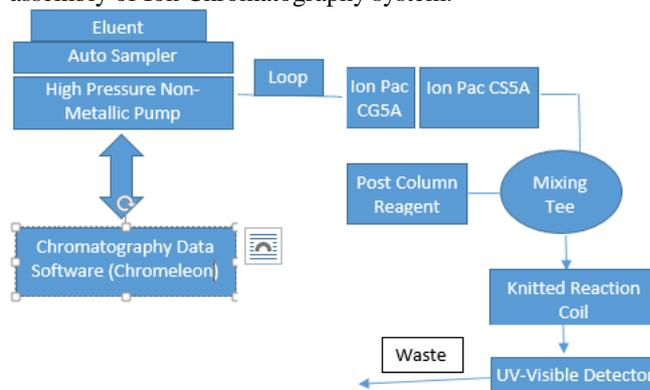
**Figure 1:** Ion Chromatography system schematic diagram for Iron (III) and Iron (II) analysis
