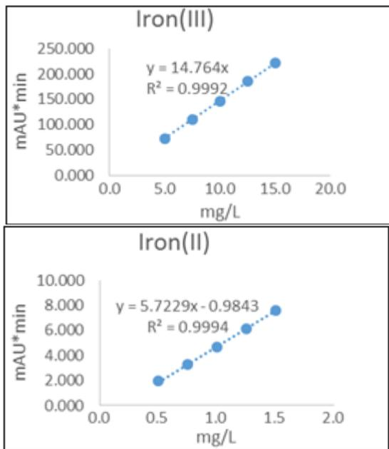
Figure 2: Linearity plot for Iron (III) and Iron(II)
