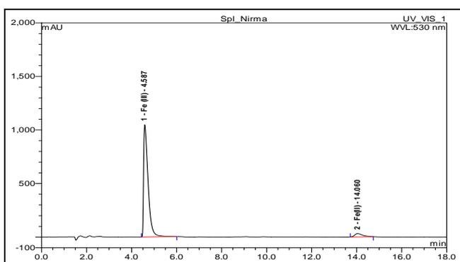
**Figure 5:** Iron Sucrose sample chromatogram (B. No. 5K10447) for Iron(III) and Iron(II) estimation.
