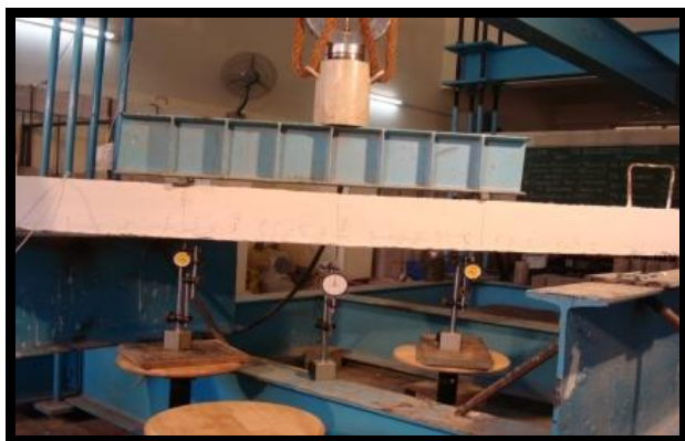
Plate: Loading Frame Test Setup
