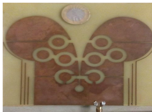
Figure 1.3: Four band Planar Reconfigurable Wideband Vivaldi Antenna
