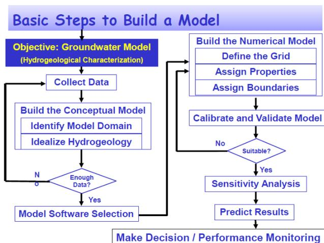
Figure 1: Flowchart for groundwater modelling process using the Visual Modflow [8]
