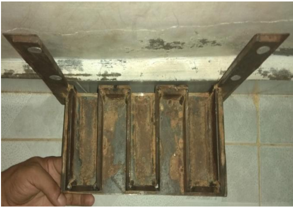
Figure 5: Rectangular Labyrinth Weir
