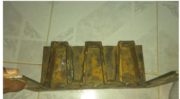
Figure 7: Trapezoidal Labyrinth Weir
