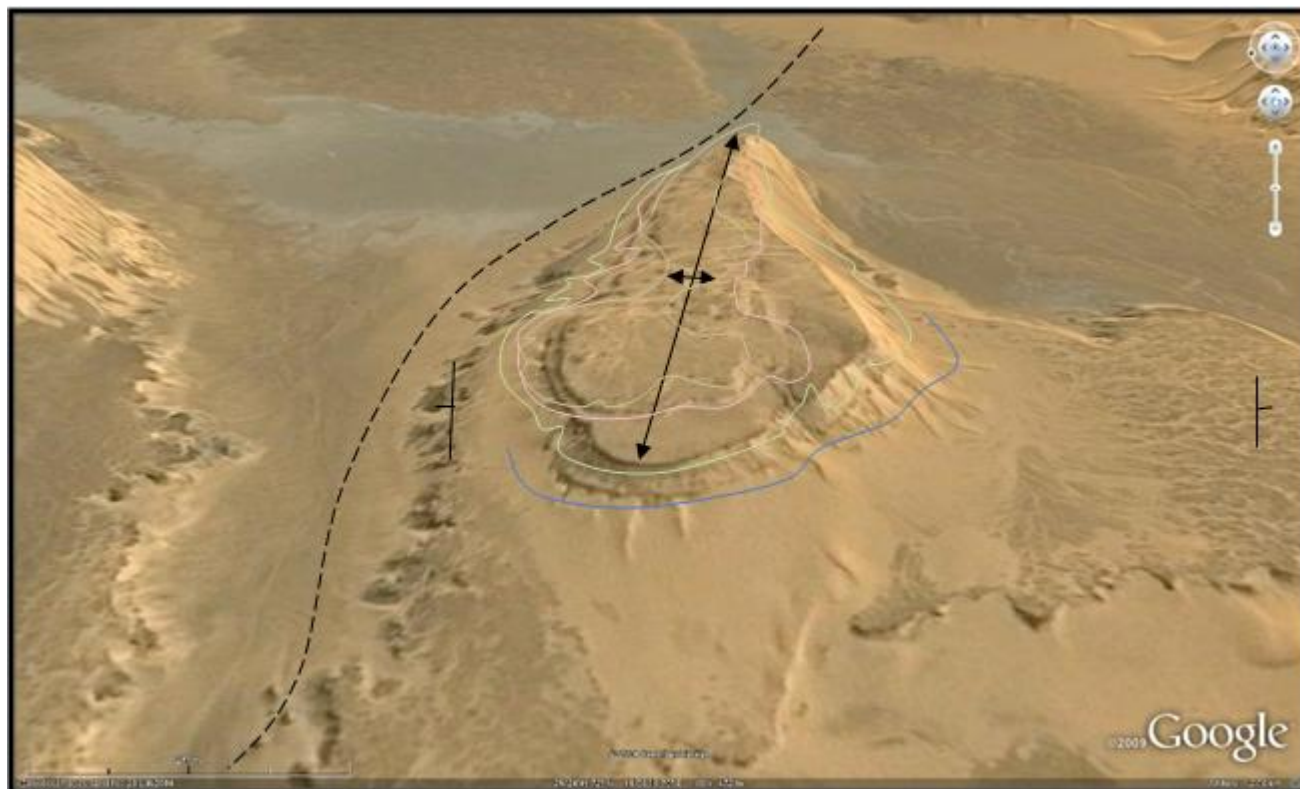
Figure 9: close-view of Google Earth, the border of Sirt Basin and Ghadamis Basin, extension fault, parallel to Hun Graben NW-SE direction, the dipping to the East (Ghadamis Basin). Vertical Exaggeration 3x.
