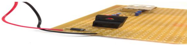
Wires from the battery holder connected
