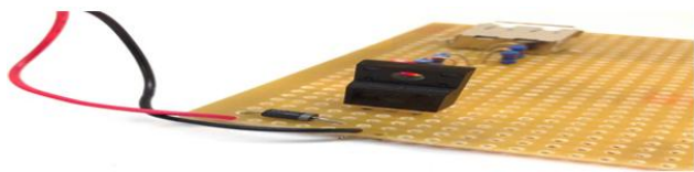
Wires from the battery holder connected
