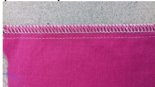
Figure 4: 5 Thread Overlock stitch picture
