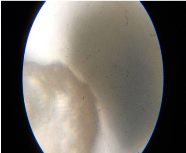
Photo 3: Microscopic Exam decay of stone, exposed/40x/ sample rao udai singh 457
