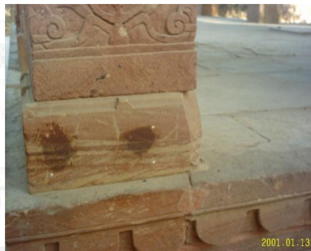
Photo 9: UPV Test on stone A. Singh Chhatri
