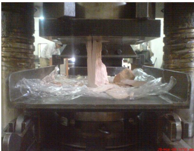
Photo 5: Stone Cylinder tested in Compression
