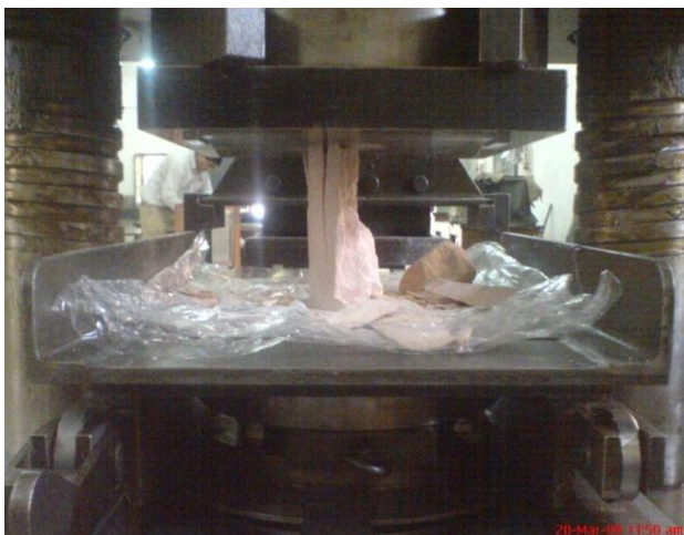
Photo 5: Stone Cylinder tested in Compression
