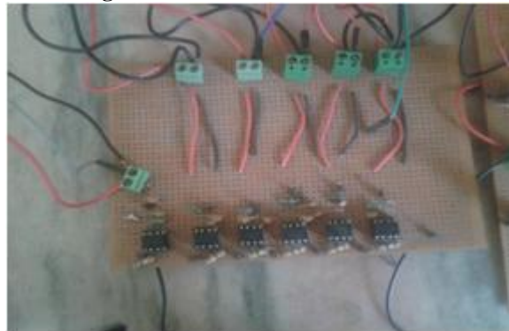
Figure 7: Hardware of pulse generation circuit
