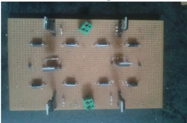
Figure 12: hardware of 7 level bridge
