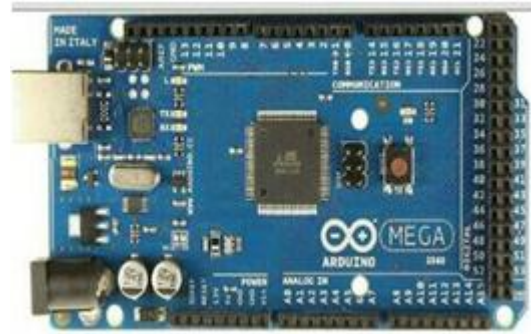
Figure 8: Diagram of microcontroller ATMEGA 2560
