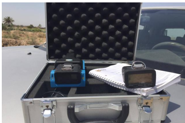
Plate 1: Device G460 use in the measurement of (CO 2 , CO, H 2 S, SO 2 , NO 2 and VOC)
