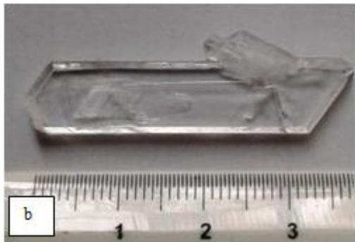
**Figure 1:** Photograph of Tartaric acid monohydrate crystal a) before and b) after recrystallization
