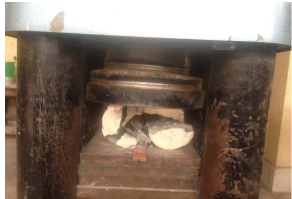
Figure 4: Tensile Splitting strength Test Set-up
