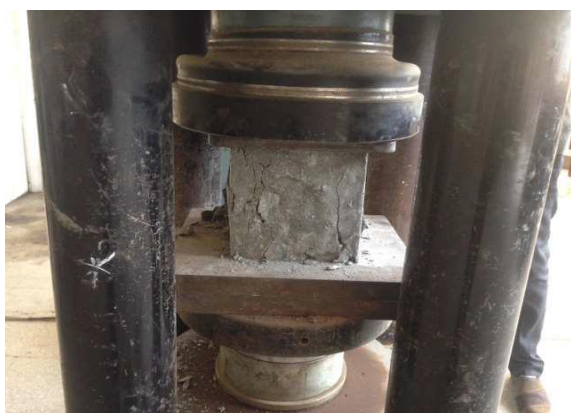
Figure 3: Compressive Strength Test Set-up
