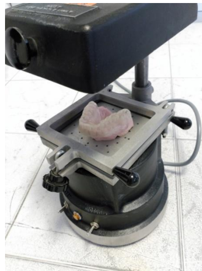
Figure 1: Dental vacuum forming machine, to make the periodontal mouthguard.
