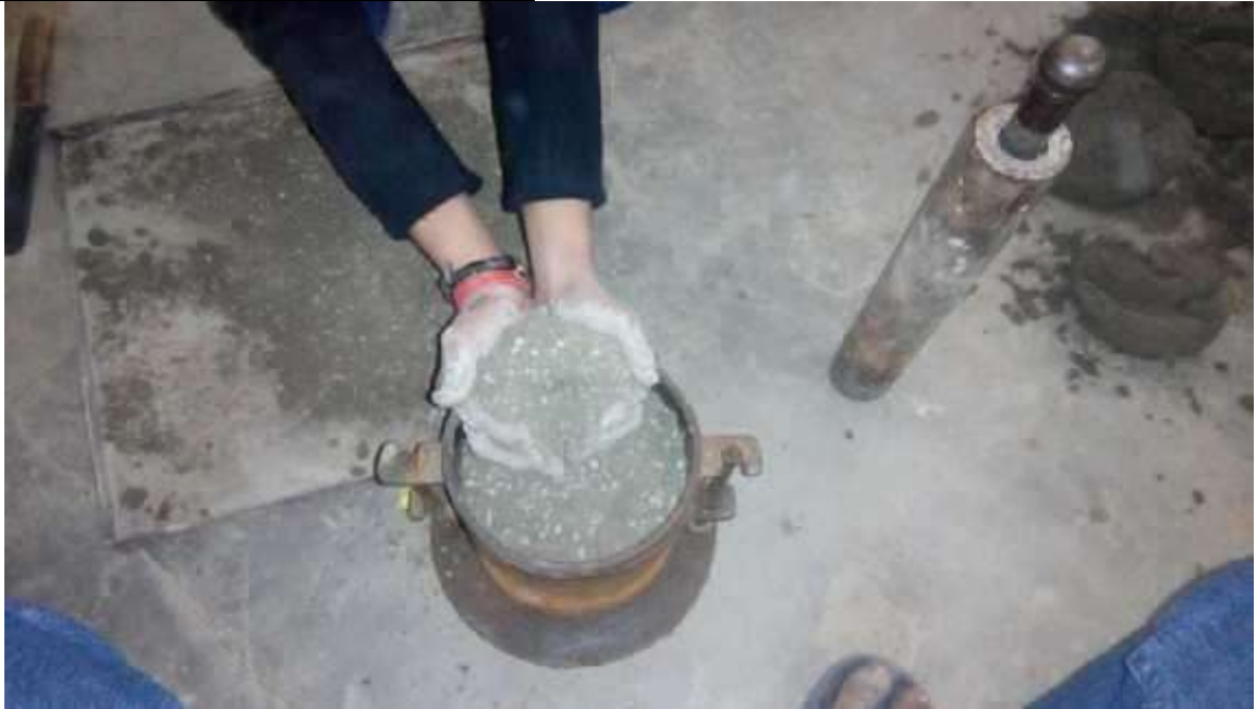
Figure 1: Filling CBR mould at optimum moisture content
