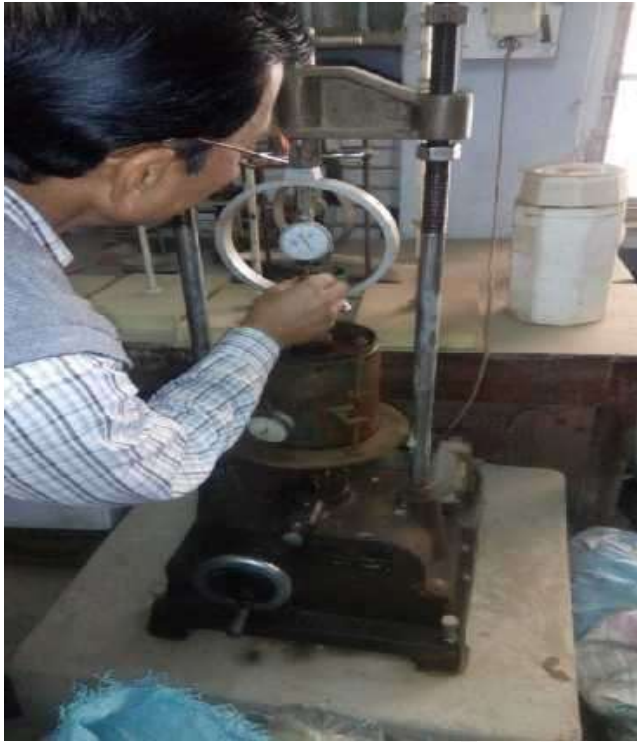
Figure 3: Setting up dial gauges before testing
