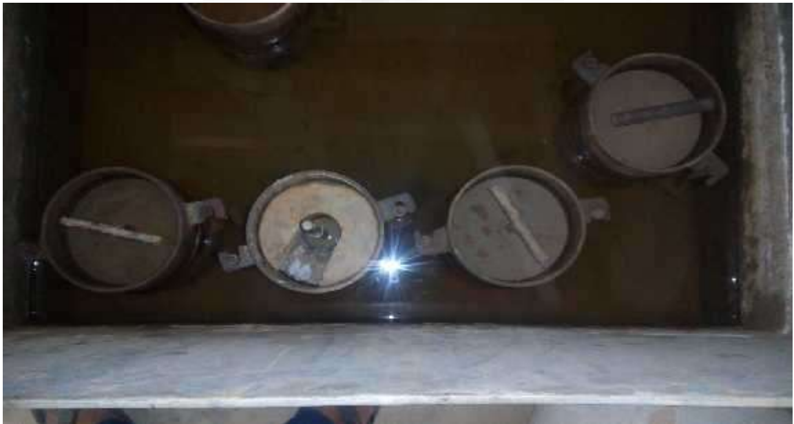
Figure 2: CBR mould kept under water for soaking of 4 days
